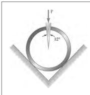
A  $12^{\circ}$  wedge is used to spread a split ring. The coefficient of static friction between the wedge and the ring is 0.30. Knowing that a force **P** of magnitude 125 N was required to insert the wedge, determine the magnitude of the forces exerted on the ring by the wedge after insertion.
