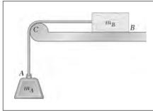
The coefficient of static friction between block *B* and the horizontal surface and between the rope and support *C* is 0.40. Knowing that  $m_A = 12$  kg, determine the smallest mass of block *B* for which equilibrium is maintained.
