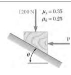
Determine whether the block shown is in equilibrium and find the magnitude and direction of the friction force when  $\theta = 25^{\circ}$  and P = 750 N.
